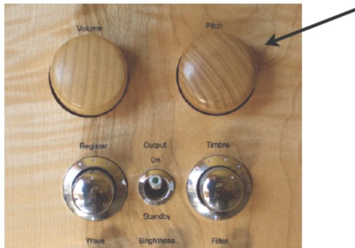
**We must turn the “Pitch” potentiometer to correctly tune our theremin.**
